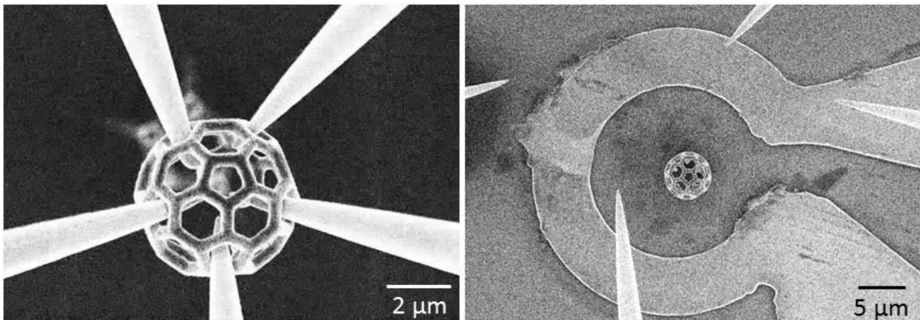
Figure 5 – Transfer of the plated structures into the microresonators: a) a buckyball grabbed by a set of micromanipulator needles and lifted from the silicon substrate; b) the structure placed in the coil microresonator and ready to be measured.
