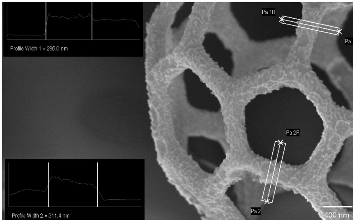
Figure 1– Close up image of the buckyball scaffold showing close-to-one aspect ratio of the composing bars.
