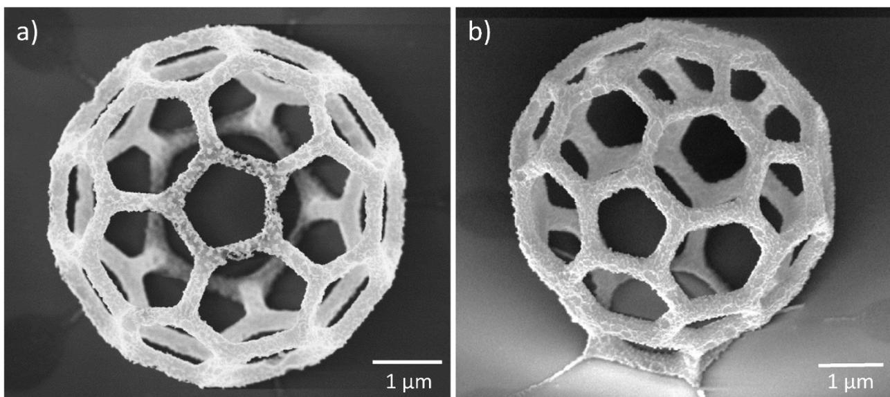
Figure 1 – SEM images of produced glassy carbon scaffold: a) top view; b) 45° tilt view.
