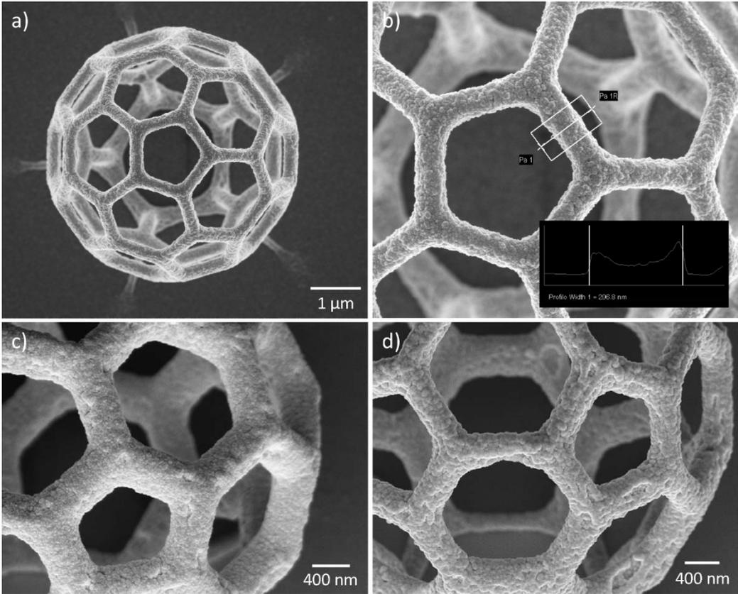
Figure 3 – SEM images of iridium coated scaffolds: a) and b) – top view; c) and d) - view at 45° angle.
